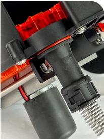
The spring adaptor cap fits on top of the switch section in the dropper assembly, with its flat side facing the switch. There is a set screw in the side of the part – screw that in to hold it in place. The screw will enter into a groove in the switch section. Again, do not over tighten!
