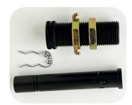
The picture above shows the dismantled dropper lower section. Once the clip is removed, the inner tube can be slid out downwards. Note the three small ball-bearings, which are caliber specific. Always dismantle over a bowl as the small balls will drop out when you remove the inner tube from the threaded body.
