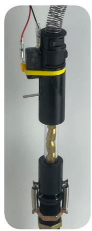
Note the position of the spring's adaptor cap as it attaches to the top of the dropper assembly. Its flat side fits snugly around the micro switch.
