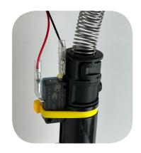
Connect the end terminals of the retractable cable to the two terminals of the micro switch, as shown. There is no polarity to be concerned with.
